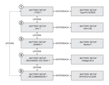
Figure 4.8 Battery Setup Menu
